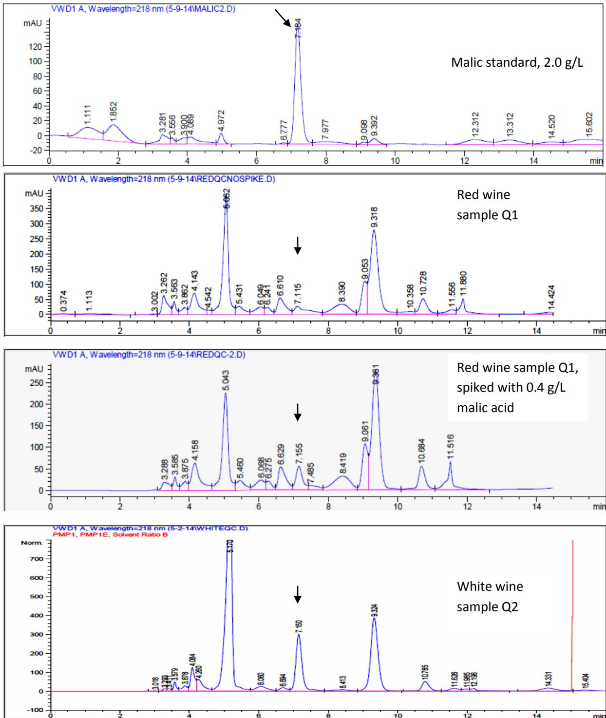
Figure 4. Chromatograms of Malic acid, RedQ1, RedQ1 spiked, and White Q2. Arrows show malic acid peak.
