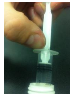
Figure 4. Withdraw the titrant from its bottle using a clean 5 mL syringe.
