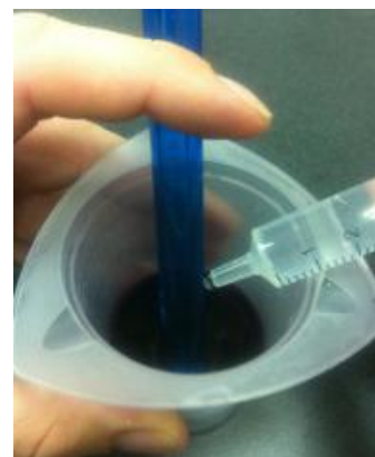
Figure 7. Manual stirring technique. Hold the electrode against the side of the titration beaker and swirl gently; add SO 2 Titrant with other hand.
