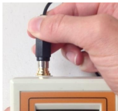
Figure 3. Be sure the Electrode attachment is secure on the RCA connector.
