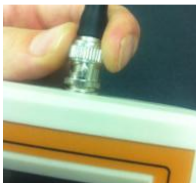
Figure 3. Be sure the Electrode attachment is screwed into place on the BNC connector.
