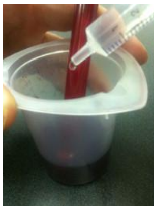
Figure 4. Manual stirring technique. Hold the electrode against the side of the titration beaker and swirl gently; add TA Titrant with other hand.
