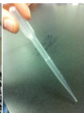
Figure 18. The transfer pipette. One full squeeze of the transfer pipette in either the Acid solution or Reactant should be approximately 2 mL.
