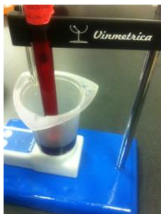
Figure 4. The Magnetic stirrer and beaker with the pH electrode inserted into the Electrode Holder to the wine sample.
