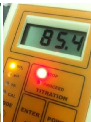
Figure 22. Once the device beeps for 15 seconds or 20 sets of "beep-beep" you are done with the titration. The red "STOP" LED will also remain lit.
