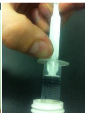
Figure 16. Withdraw the titrant from its bottle using a clean 5 mL syringe. If you are using the glass burette, use the syringe to fill it.
