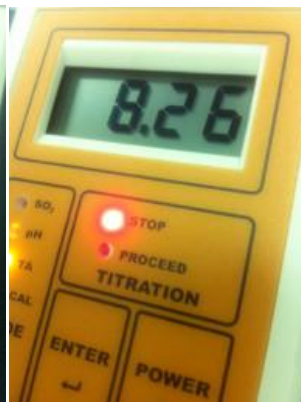
Figure 26. Once the pH arrives at or passes 8.20 you are done with the titration. The red "STOP" LED will be lit and the instrument will be beeping
