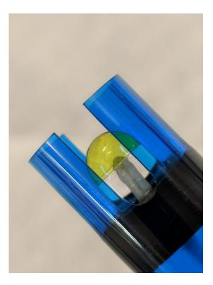
Side view of a pH electrode. The glass bulb is the pH sensing element. Inside is a silver/silver chloride electrode and a potassium chloride reference buffer solution
