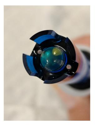
Bottom view of a pH electrode. The glass bulb is the pH sensing element. On either side are the ceramic frits (reddish from use in red wines) of the reference junction that provide contact of the test solution to the reference electrode inside.
