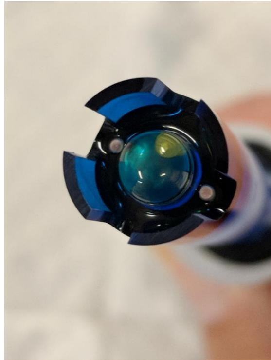
Bottom view of the pH electrode. The glass bulb is the pH sensing element. On either side are the ceramic frits (reddish from use in red wines) of the reference junction that provide contact of the test solution to the reference electrode inside.
