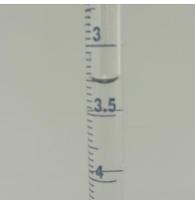
Figure 10. The Meniscus of the water column. This curve is formed because of interactions of water with the glass burette. We recommend measuring the titrant volume from the bottom of the meniscus. In the picture the value is about 3.27 mL.
