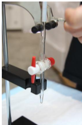
Figure 7. The glass burette tip can be placed just outside the Electrode Holder's front slot for accurate titrations.
