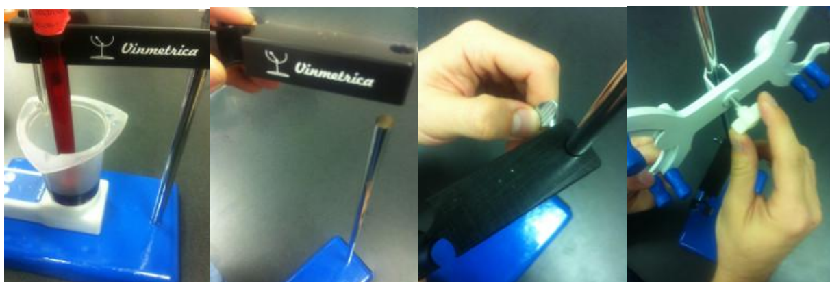
Figure 1. The Magnetic stirrer and beaker with the pH electrode inserted into the Electrode Holder to the wine sample.
