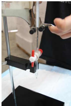
Figure 6. The burette sits firmly between the notches of the four spring arm knobs of the Double Burette Clamp.
