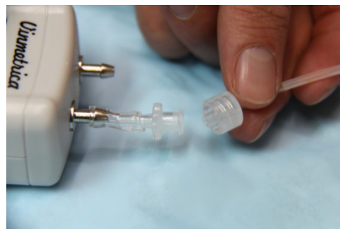
Figure 2. Disconnecting the vial insertion assembly
