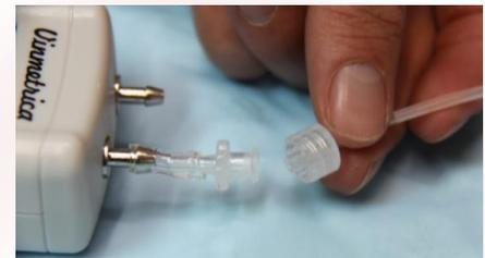
Figure 1. Unscrew the Luer Lock connector.
