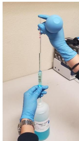
*Illustration 1: step d. controlling the speed of drain from the pipette.*
