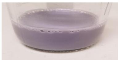
*Fig. 2: The color of the reaction when titration is almost done*
